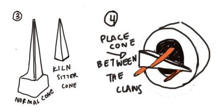
When the kiln reaches the correct temp it will melt the cone and shut it off automatically. There are a couple other fail safes, but this is the most reliable.
