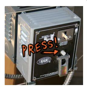
That's the button that gives the kiln the okay to surge electricity through the elements, but it's not on yet. Then go to the little stand that's next to and connected to the kiln, and press the on button. Now the Kiln is ON.
